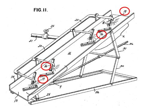
Once the shrimp had passed through the "slitter," the vein was exposed, but only sometimes removed.<sup>30</sup> To complete the vein removal, the shrimp were passed through a tumbler which would hook the vein and remove it.31 The "deveiner" patent elements, as depicted by Figures 1 and 11 of U.S. Patent No. 2,825,927, below, included: (1) a supporting member (25); (2) a "lip" (24); and (3) a "means" for moving the shrimp (water jets, not pictured). <sup>32</sup>
